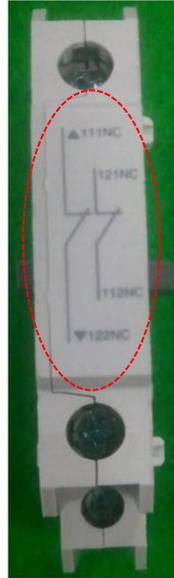
Before assembly, check if MC & UR are on the right direction.
