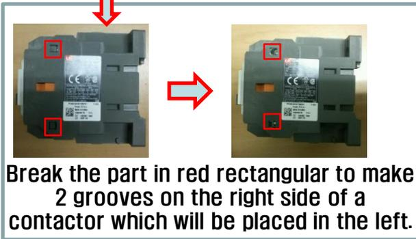
Break the part in red rectangular to make 2 grooves on the right side of a contactor which will be placed in the left.
