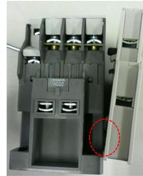
Match hooks on UR-02 with grooves on the side of a MC
