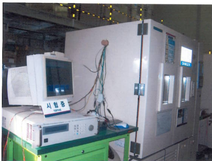
Photo. 1. test arrangement of outer chamber - Programmable power source and temperature chamber
